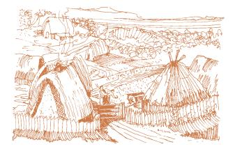
Original settlement houses - timber posts and frames with wattle and daub walls and thatched roofs
